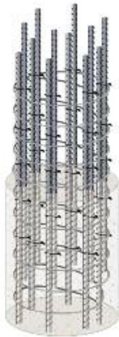
Lap splicing inhibits concrete consolidation
